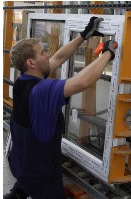
USE THE GLAZING HAMMER TO ATTACH THE GLAZING SLAT (BEAD).
