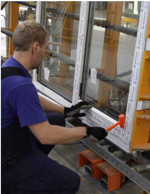
USE THE GLAZING HAMMER TO ATTACH THE GLAZING SLAT (BEAD).
