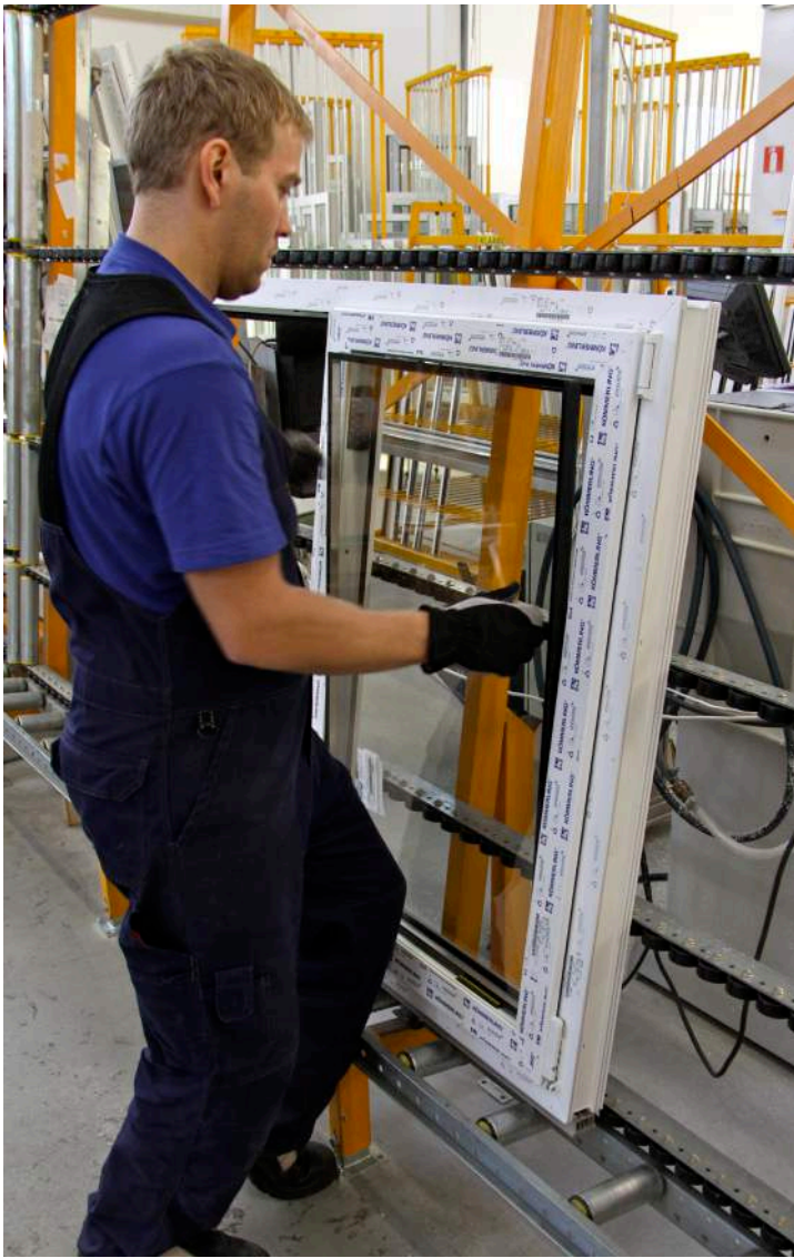
INSERT GLASS AND USE THE GLAZING BLADE AND BLOCKS TO FIXATE THE POSITIONING OF THE GLASS IN THE FRAME
